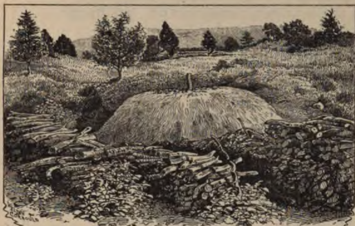
A Charcoal Pit ready for "firing"
